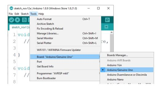
The port to which the microcontroller board is connected has to be selected. Go to: *Tools > Port > {port name goes here}*
